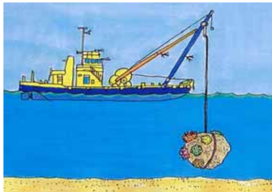
Fig. 5-3 . Transport of base rock collected (Hirara Harbor Construction Office 2002)
